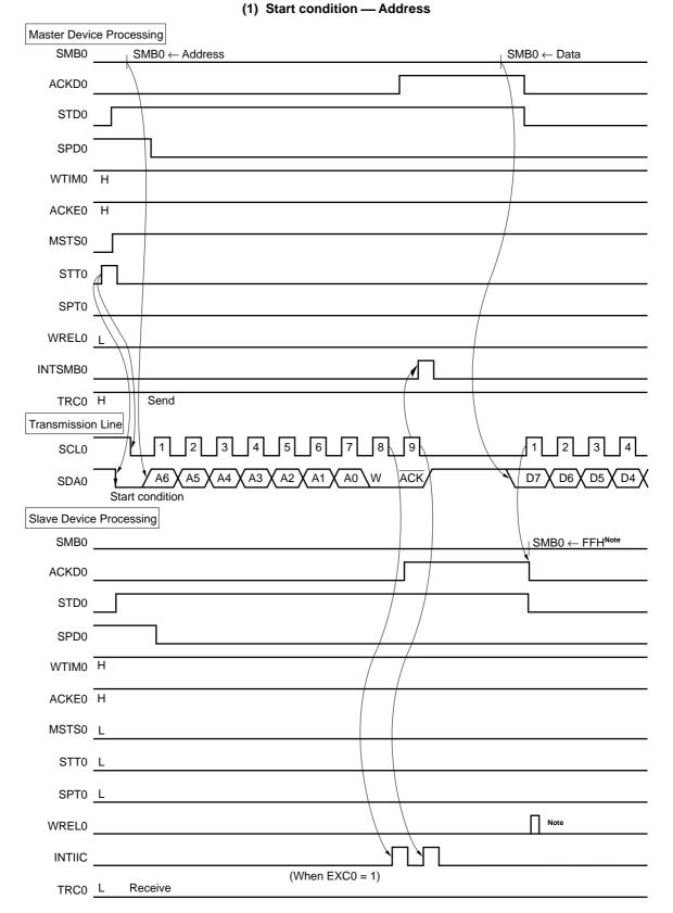
Figure 15-20. Master  $\rightarrow$  Slave Communication Example (When 9-Clock Wait is Selected for Both Master and Slave) (1/3)
