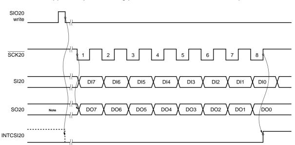
Figure 14-11. 3-Wire Serial I/O Mode Timing (2/7)
