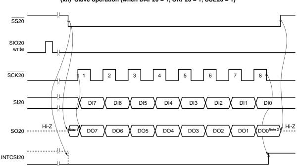
Figure 14-11. 3-Wire Serial I/O Mode Timing (7/7)
