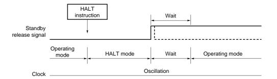
**Remarks 1.** The broken line indicates the case where the interrupt request that has released standby mode is accepted.
