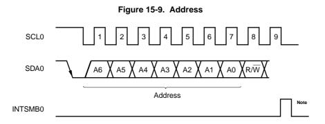
Note If other than a local address or extension code is received during slave operation, INTSMB0 is not issued.
