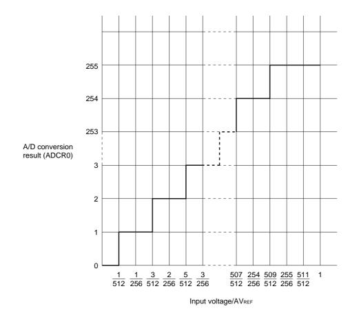
Figure 12-5. Relationship between Analog Input Voltage and A/D Conversion Result
