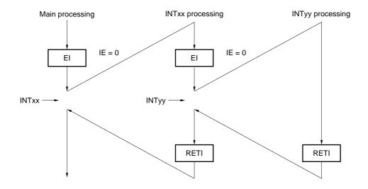
During interrupt INTxx servicing, interrupt request INTyy is accepted, and a multiple interrupt is generated. An EI instruction is issued before each interrupt request acceptance, and the interrupt request acceptance enable state is set.
