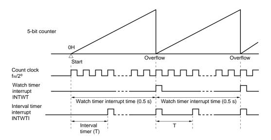
Figure 10-3. Watch Timer/Interval Timer Operation Timing
