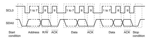
The start condition, slave address, and stop condition are output by the master.
