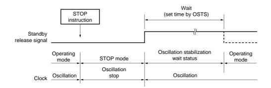
**Remark** The broken lines indicate the case where the interrupt request that has released standby mode is accepted.
