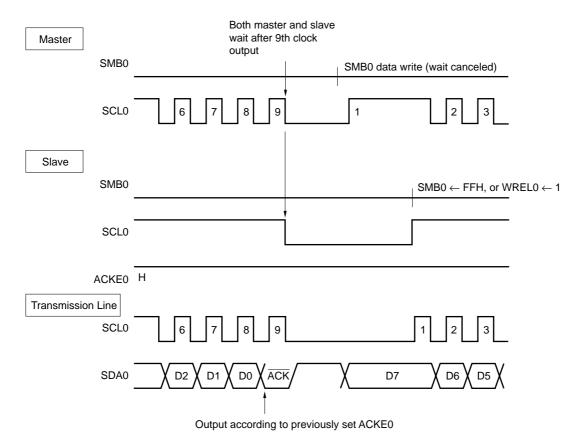
Remark ACKE0 : SMB control register 0 (SMBC0) bit 2 WREL0 : SMB control register 0 (SMBC0) bit 5
