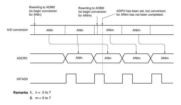
Figure 12-11. A/D Conversion End Interrupt Request Generation Timing
