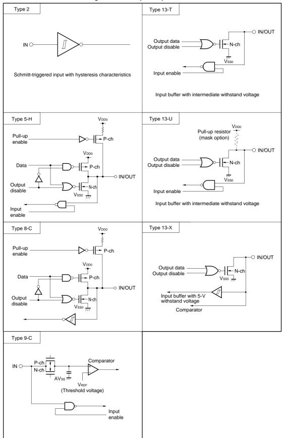
Figure 4-1. Pin Input/Output Circuits
