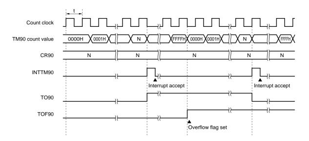
Figure 8-6. Timing of Timer Interrupt Operation
