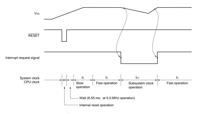
Figure 7-8. Switching between System Clock and CPU Clock
