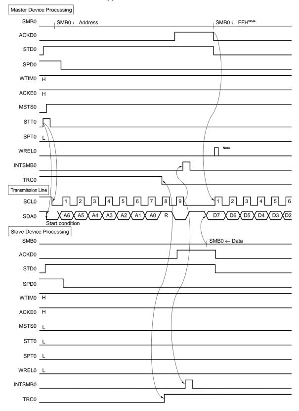
Figure 15-21. Slave  $\rightarrow$  Master Communication Example (When 9-Clock Wait is Selected for Both Master and Slave) (1/3)
