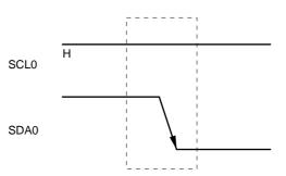
The start condition is output when SMB control register 0 (SMBC0) bit 1 (STT0) is set to 1 in the stop condition detection status (STD0: SMB status register 0 (SMBS0) bit 1 = 1). Moreover, when the start condition is detected, SMBS0 bit 1 (STD0) is set to 1.
