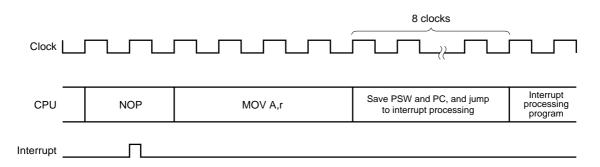
If an interrupt request flag ( $\times$ IF) is set at the last clock of the instruction, the interrupt acceptance processing starts after the next instruction is executed. Figure 17-12 shows an example of the interrupt acceptance timing for an interrupt request flag that is set at the second clock of NOP (2-clock instruction). In this case, the MOV A,r instruction after the NOP instruction is executed, and then the interrupt acceptance processing is performed.
