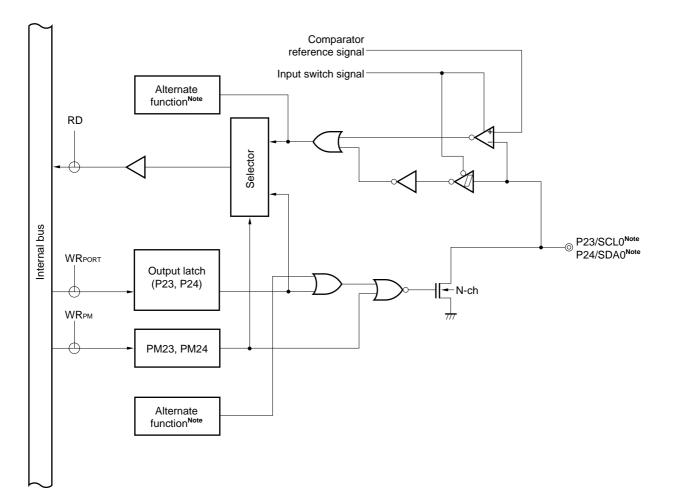
Figure 6-7. Block Diagram of P23 and P24
