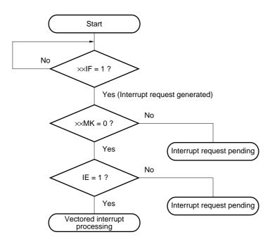
Figure 17-10. Interrupt Request Acceptance Processing Algorithm
