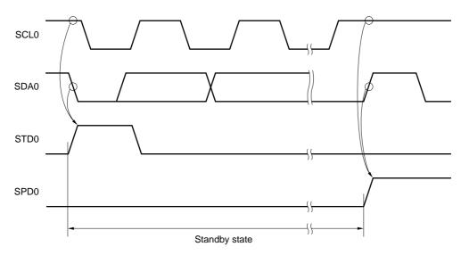
Figure 15-16. Communication Reservation Received Timing
