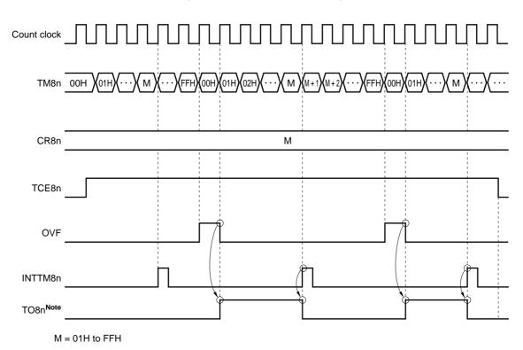
Figure 9-12. PWM Output Timing
