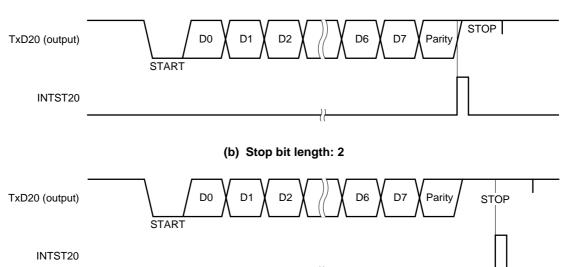
Caution Do not rewrite to asynchronous serial interface mode register 20 (ASIM20) during a transmit operation. If the ASIM20 register is rewritten to during transmission, subsequent transmission may not be performed (the normal state is restored by RESET input).
