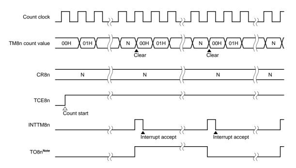
Figure 9-11. Square Wave Output Timing
