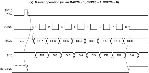
Figure 14-11. 3-Wire Serial I/O Mode Timing (6/7)
