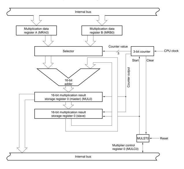
Figure 16-1. Block Diagram of Multiplier
