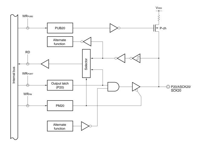
Figure 6-4. Block Diagram of P20
