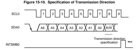
Note If other than a local address or extension code is received during slave operation, INTSMB0 is not issued.
