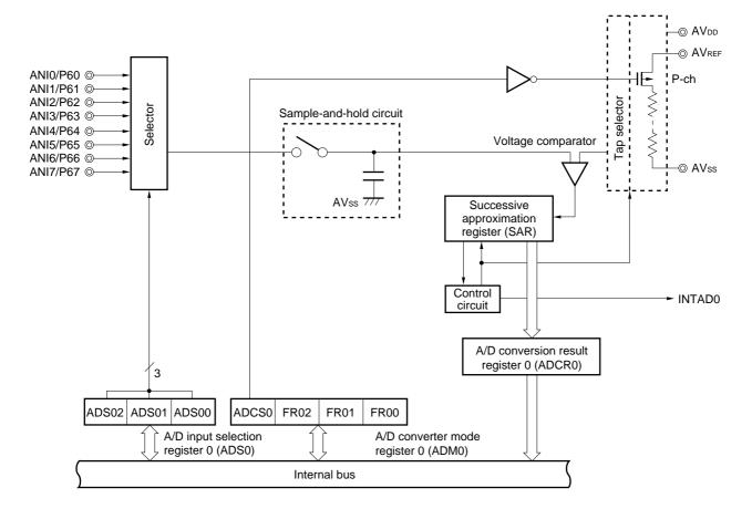
Figure 13-1. Block Diagram of 10-Bit A/D Converter
