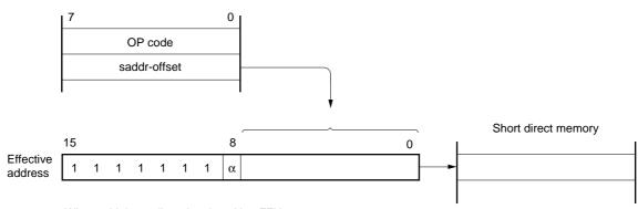
When 8-bit immediate data is 20H to FFH,  $\alpha = 0$ . When 8-bit immediate data is 00H to 1FH,  $\alpha = 1$ .
