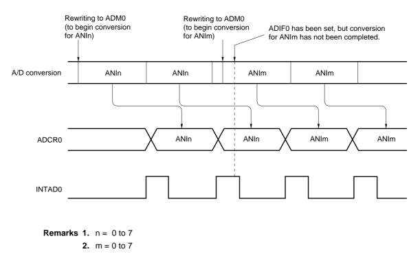
Figure 13-11. A/D Conversion End Interrupt Request Generation Timing
