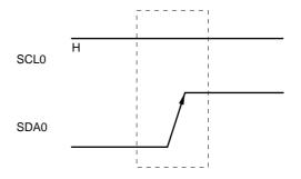
A stop condition is generated when bit 0 (SPT0) of SMB control register 0 (SMBC0) is set to 1. If, when a stop condition is detected, bit 0 (SPD0) of SMB status register 0 (SMBS0) and bit 4 (SPIE0) of SMBC0 are set to 1, INTSMB0 is generated.
