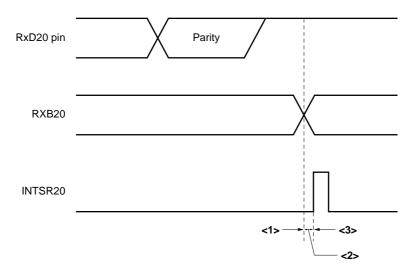
When RXE20 is set to 0 at a time indicated by <1>, RXB20 holds the previous data and INTSR20 is not generated.
