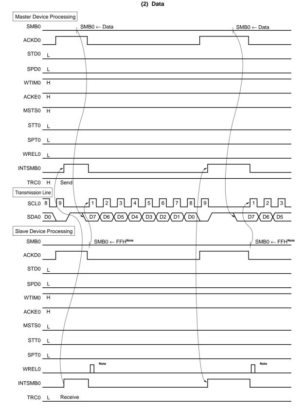
Figure 15-20. Master  $\rightarrow$  Slave Communication Example (When 9-Clock Wait is Selected for Both Master and Slave) (2/3)
