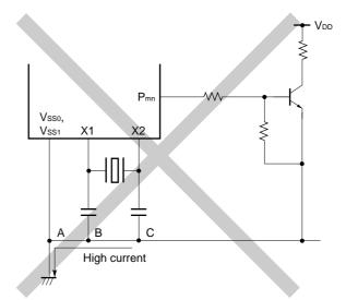
**Remark** When using the subsystem clock, read X1 and X2 as XT1 and XT2, respectively, and connect a resistor to the XT2 pin in series.
