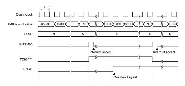
Figure 8-8. Timer Output Timing
