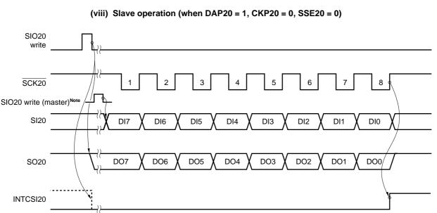
Figure 14-11. 3-Wire Serial I/O Mode Timing (5/7)
