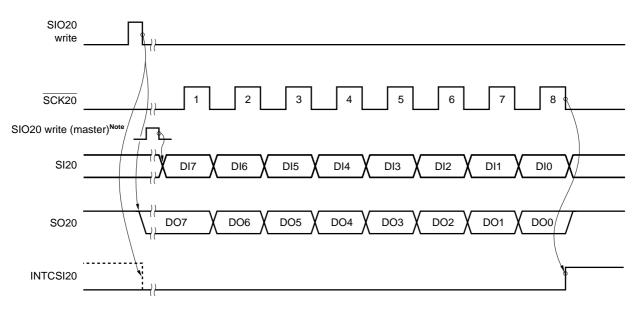
**Note** The data of SI20 is loaded at the first rising edge of  $\overline{SCK20}$ . Make sure that the master outputs the first bit before the first rising of  $\overline{SCK20}$ .
