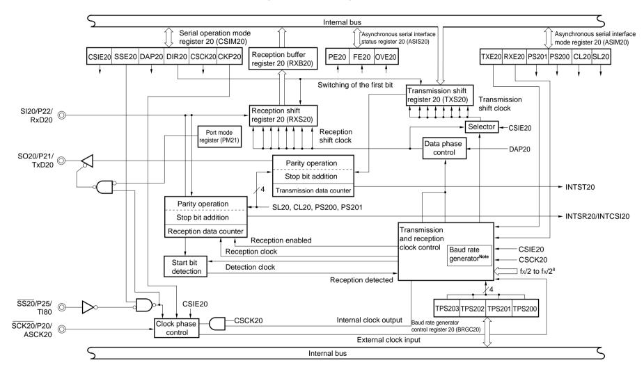
Figure 14-1. Block Diagram of Serial Interface 20
