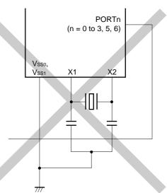
(d) Current flowing through ground line of oscillator (potential at points A, B, and C fluctuates)
