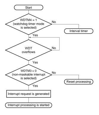
Figure 17-7. Flowchart from Non-Maskable Interrupt Request Generation to Acceptance
