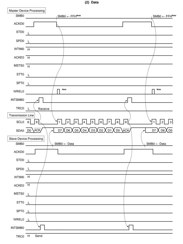
Figure 15-21. Slave  $\rightarrow$  Master Communication Example (When 9-Clock Wait is Selected for Both Master and Slave) (2/3)
